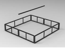
5. Ensure that cross bar is fully inserted and level with the stage frame.
